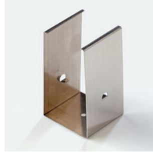
KKCP-17 Lock clip (allow 2 per metre/40in) S/Steel finish L25/W26.1/H45mm (L0.98/W1.03/H1.77")
